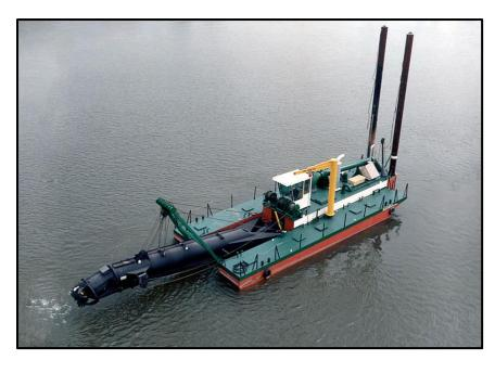
The "Jumeirah Bay" is a Cutter Suction Dredger from the IHC Beaver line built in 1992. Gulf Cobla completely refurbished this dredger in 2014, resulting in her current practical new state.
